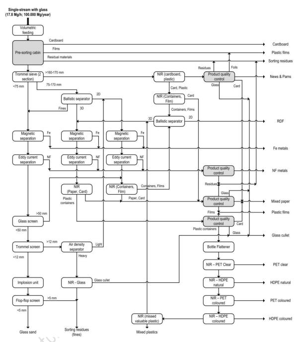
Figure 2. Example of sorting plant (material recovery facility) managing a single-stream commingled input of glass, metal, paper and cardboard, and plastic. Arrows represent conveyor belts. OCC: old corrugated cardboard; HDPE: high-density polyethylene; PET: polyethylene terephthalate. Taken from (Cimpan et al., 2015).
