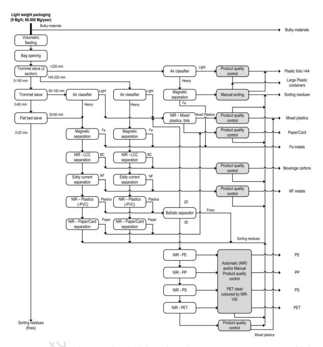
Figure 3. Example of sorting plant for lightweight packaging, i.e. managing an input of light packaging composed of plastic, metal, and beverage cartons (including other composite). BC: beverage cartons; OCC: old corrugated cardboard; HDPE: high-density polyethylene; LCC: liquid carton containers; NIR: near-infrared; PE: polyethylene; PET: polyethylene terephthalate; PP: polypropylene; PS: polystyrene; PVC: polyvinyl chloride; Taken from (Cimpan et al., 2015).
